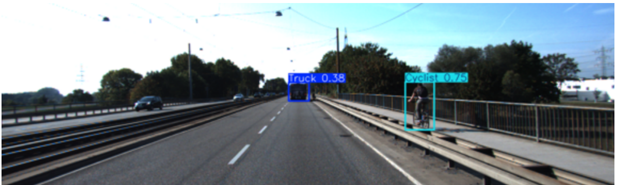
Figure 4.3: YOLO Global Model: After Federated Averaging, the model successfully detects BOTH the Truck and the Cyclist in the same scene.
