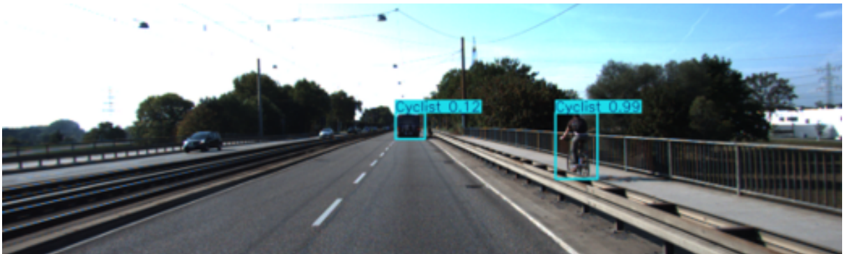
Figure 4.2: YOLO Client 2 (Cyclist Specialist): The model detects the Cyclist but ignores the Truck, treating it as background.
