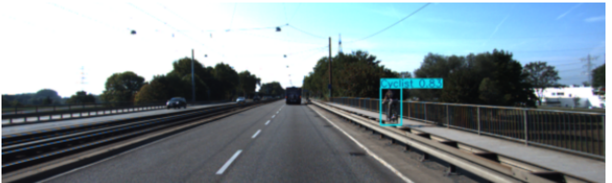
Figure 4.8: RT-DETR Client 2: The Cyclist specialist ignores the truck entirely but places a high-confidence bounding box on the cyclist.
