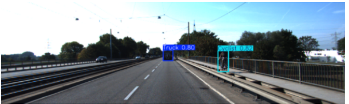
Figure 4.9: RT-DETR Global Model: The aggregated model demonstrates superior recall, detecting both the distant Truck and the Cyclist that the individual clients missed or detected with lower confidence.
