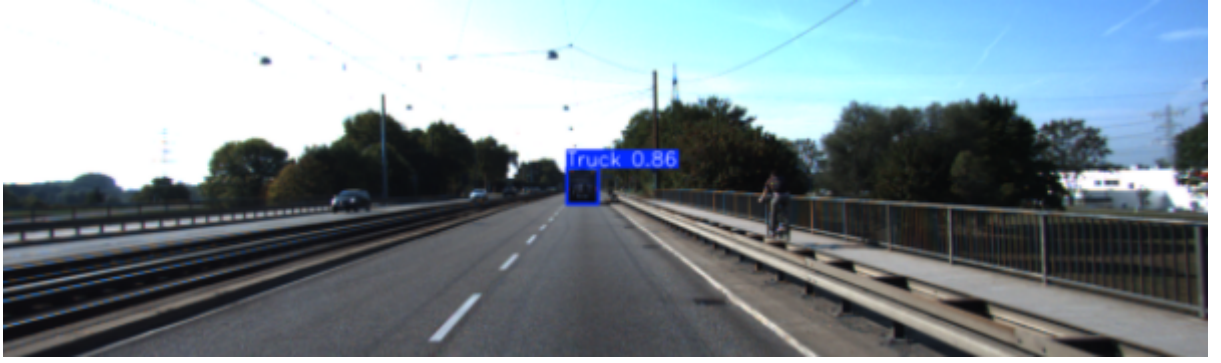
Figure 4.7: RT-DETR Client 1: The Truck specialist successfully bounds the large vehicle but fails to detect the cyclist on the right.
