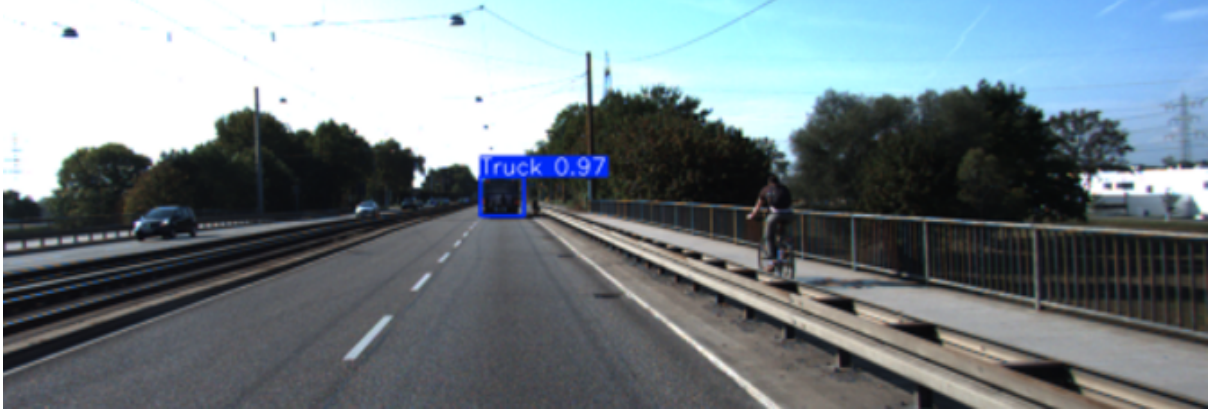
Figure 4.1: YOLO Client 1 (Truck Specialist): The model correctly identifies the Truck with high confidence but completely misses the Cyclist.
